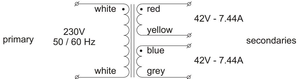
serial operation to double the secondary voltage
