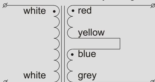
parallel operation to double the secondary current
